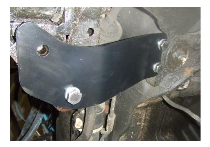
**STEP 3)** After the plates are in place, bolt on the main <u>crossmember</u> bar. Use the OE nuts and <u>no washers</u>. Using a washer only takes away from thread engagement here.
