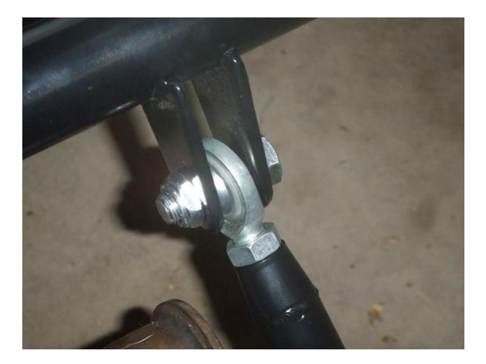
At the rear connection of each parallel arm, slide the aluminum bushing into the heim so that the step portion is between the heim and the plate (*NOTE: these ship already installed in the heim – just remove the zip tie*). Use the 65mm bolts and washers to bolt these up. Once they're attached, you can torque down all six bolts on the two k-member plates.
