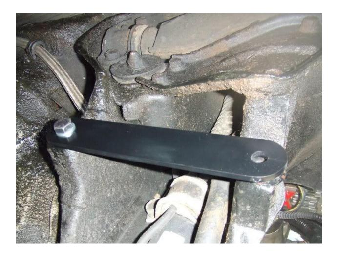
Next is the 4-bolt drivers side plate. At the rear of the plate, fit the edge of it up under the edge of the rubber bushing, and then lay the plate flat. Install the 40mm bolts finger snug - do not fully tighten these yet either.
