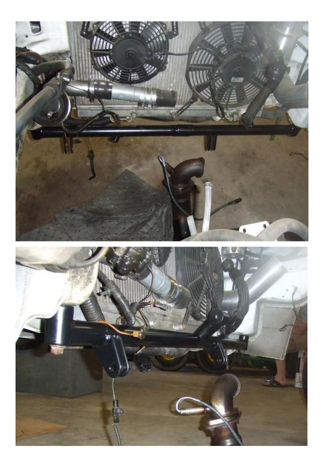
**STEP 4)** Now onto the parallel bars. Use the supplied 1/2" bolts and nuts to attach them on the <u>crossmember</u> end first. No washers needed here either. You can fully tighten these nuts/bolts now.
