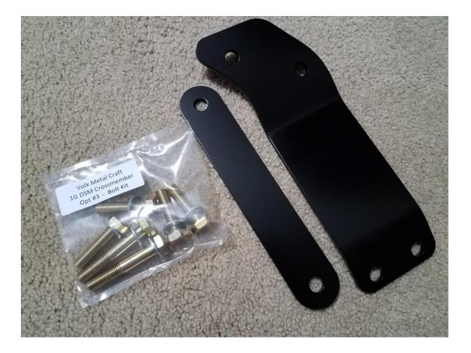
Start with the 2-hole passenger side plate. Install it in place with only the rear bolt snugged up with your fingers. Do not tighten this bolt up just yet.
