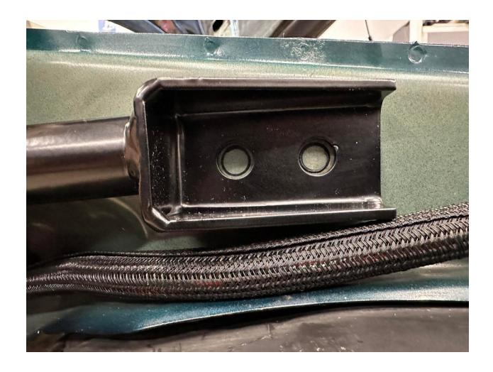
**Step 4:** Time to drill!! Center punch your two holes and drill using a 11mm or 7/16" size drill bit. Next, locate the hole use to attach the wiring. Unclip and use this as your center and create a 1- 3/8" hole using a hole saw or stepped bit.
