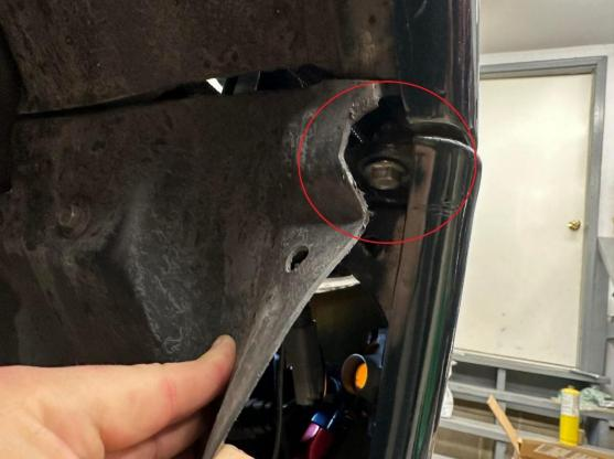
**Step 3:** Next step is to mock up the fender brace to mark holes to drill. To do this, you'll be removing the bolts from the door hinge. *PRO TIP:* Wedge a shop towel between the door and frame to keep the door from moving and to prevent a paint chip. Mock up the fender brace, and trace your holt holes onto the chassis.
