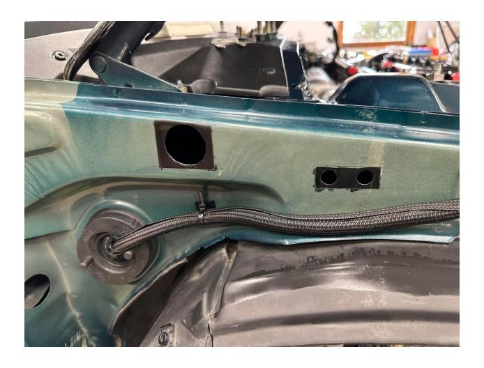
Step 5: Install the fender brackets onto the door hinges. The forward part should have the holes lines up with the ones you drilled. Feed the brackets in through the 1-3/8" hole and align it with the fender brace, and install the bolts.
